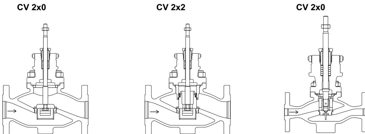
Pic.1: Flow direction for two-way valve with V-ported or contour plug
