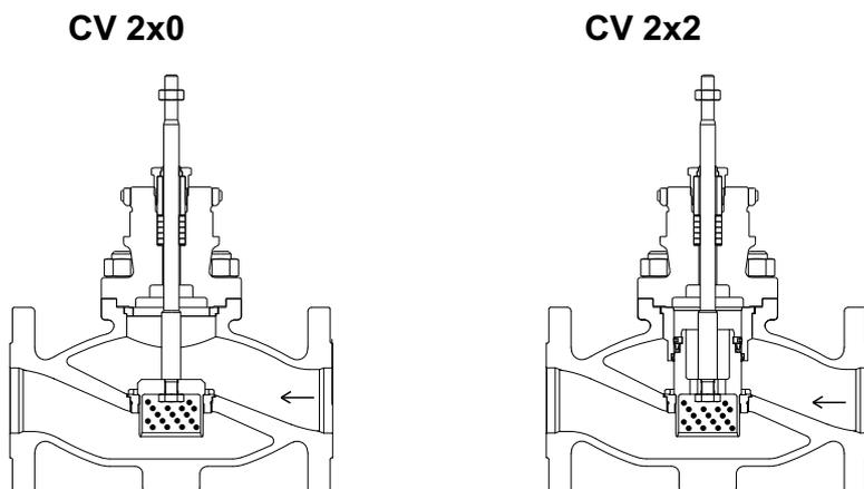
Pic.2: Flow direction for valve with perforated plug
