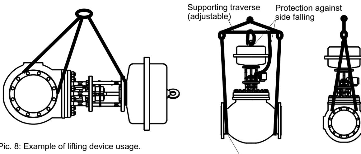
Pic. 8: Example of lifting device usage.
